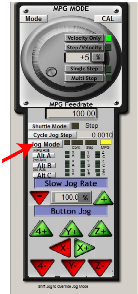
Figure4-3. Change to MPG mode on MPG panel
