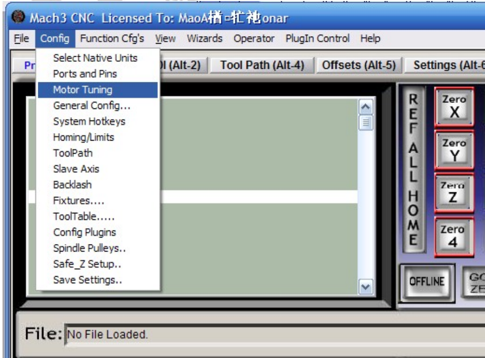
Figure4-5. Motor operating parameter setting menu entry
